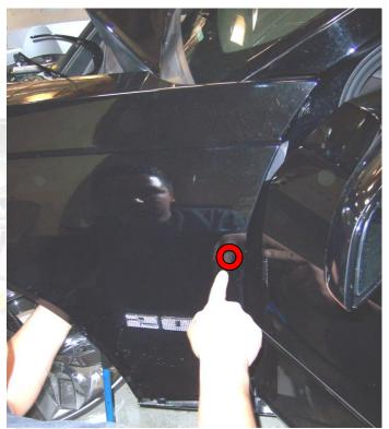
Pull on the wheel well (by front bumper), and remove (1) 10mm bolt and loosen (2) 10mm nuts; note you will need a long socket to loosen the nuts.
