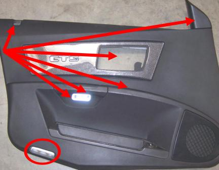
After removing the door panel you will be able to remove the door catch by removing the speaker.
