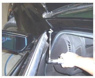
Open the door and remove (1) 10mm bolt from the top, between the door and the windshield pillar.
